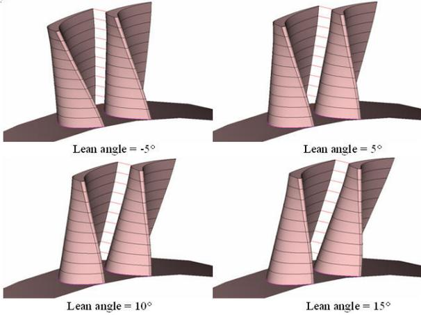
Fig. 2 Sketches of lean blades in rotor.
