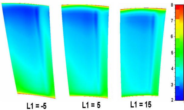
Fig. 6 Entropy at outlet of stator ( $J/(kg \cdot k)$ ).
