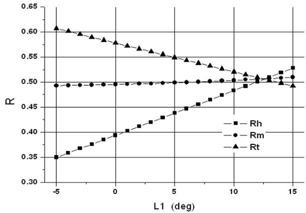
Fig.9 Reaction in hub, mean and tip region.
