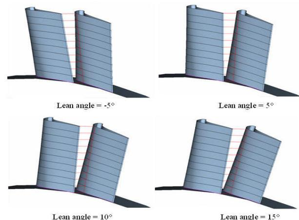
Fig. 1 Sketches of lean blades in stator.
