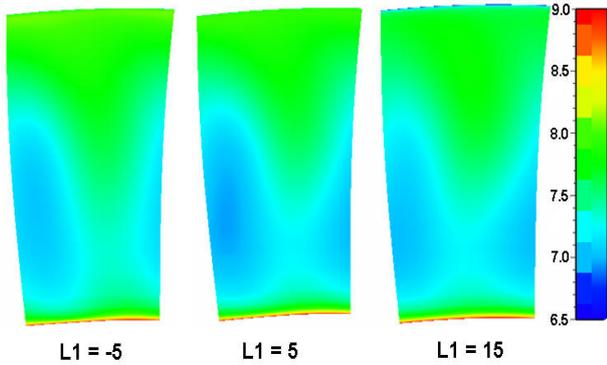
Fig. 7 Entropy at outlet of rotor ( $J/(kg \cdot k)$ ).
