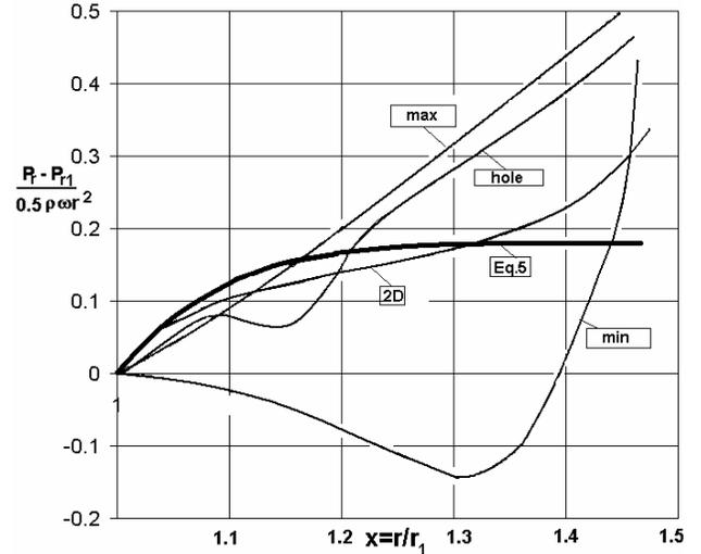
**Figure 11. Pressure factor distribution in the fore cavity at reference pressure 16.3 MPa. 3D- instantaneous values along radiuses crossing balance hole axis (hole), vortex center (min), and maximal pressure zone (max); 2D - along radius; Eq.5 - 1D analysis based on equations (5-8).**
