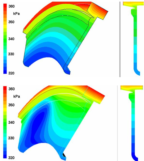
Figure 3. Pressure distribution with 3D (left) and 2D (right) models of the fore near-disk cavity. Above -  $P_{op}=1\text{MPa}$  , below  $P_{op}=16.3\text{MPa}$
