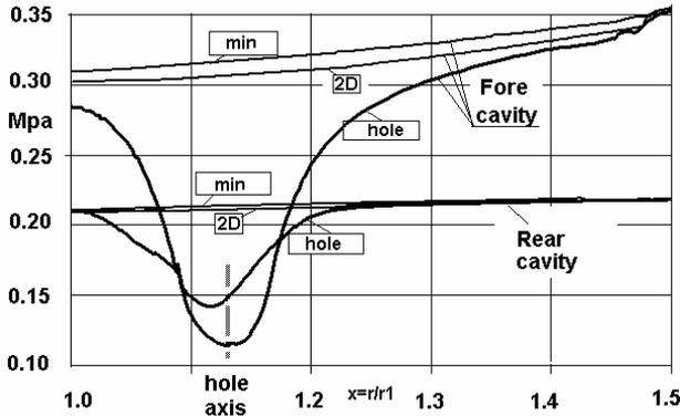
**Figure 10. Distribution of relative static pressure along radii crossing balance hole axis (hole), vortex center (min) in 3D model and along radius in 2D model for fore and rear cavities at reference pressure 1.0 MPa**
