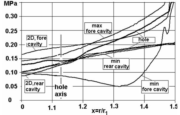
Figure 9. Distribution of relative static pressure along radii crossing balance hole axis (hole), vortex center (min) and zone of maximal pressure (max) in 3D model and along radius in 2D model for fore and rear cavities at reference pressure 16.3 MPa
