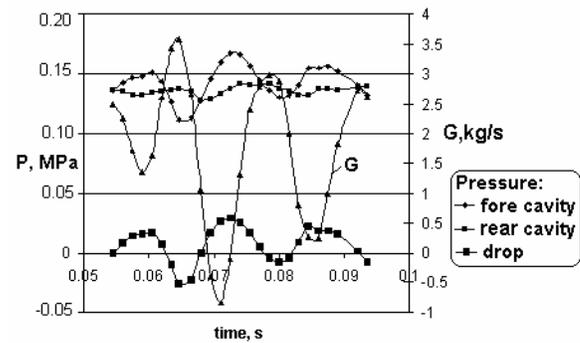
Figure 5. Static pressure difference in fore and rear cavities along surface of annulus enveloping balance holes. G - Steam flow rate through balance holes.
