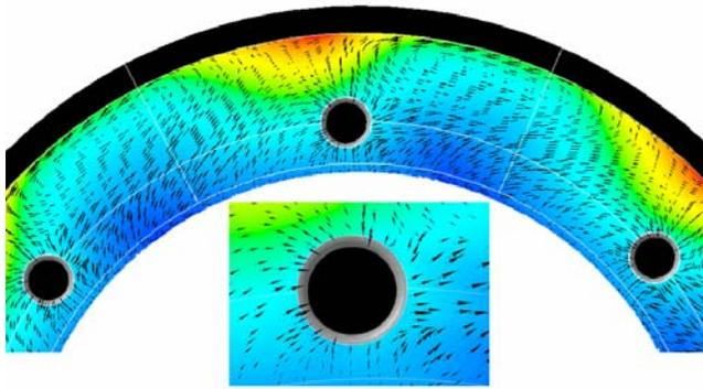
**Figure 7. Flow near fore surface of disk at minimal pressure drop and respective maximum of through holes flow rate**
