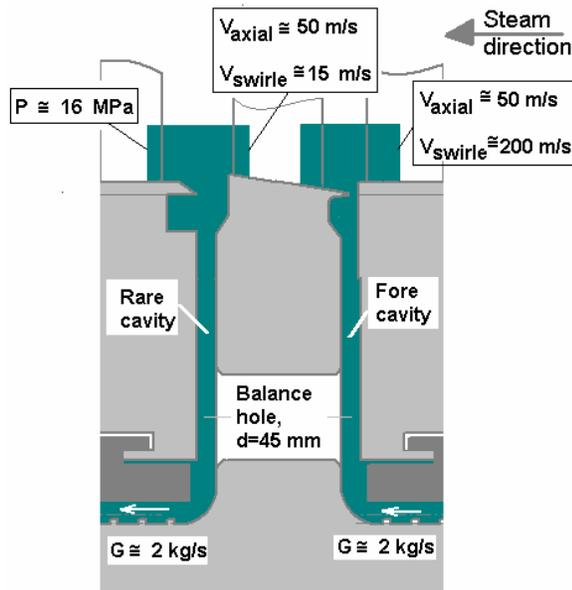
**Figure 1. Model of the disk cavities (green sectors) channelled with balance holes (white sector)**
