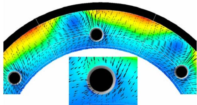
Figure 6. Flow near fore surface of the disk at maximal pressure drop and respective minimum of through holes flow rate
