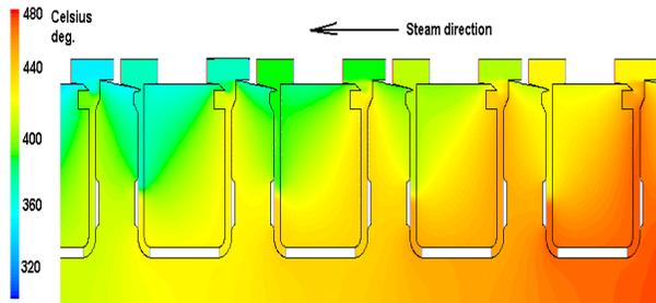
**Fig. 12 Fragment of temperature distribution of rotor and diaphragms**
