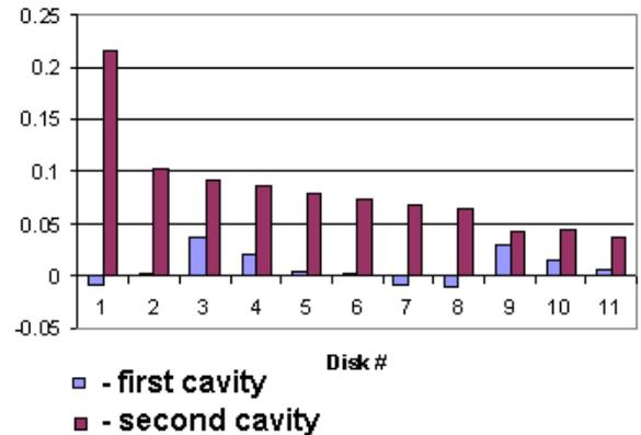
**Fig. 10 Relative windage losses in disks - friction loss normalized by total frictional loss in all disks**
