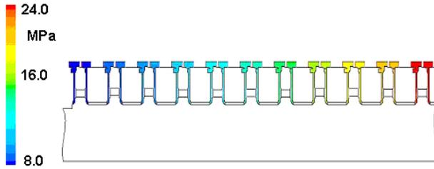
**Fig. 8 Static pressure distribution of secondary steam**
