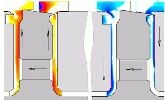
**Fig. 3 Radial velocity in cavities around disk of the 4<sup>th</sup> stage. (a) - positive radial velocity in the range of 0 (blue) – 15 (red), m/s; (b) - negative velocity in the range of (-25) (blue) – 0 (light blue), m/s**
