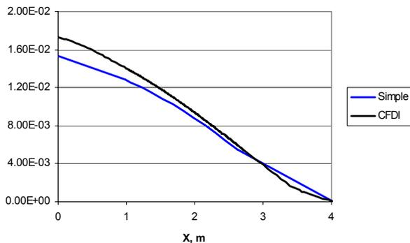
**Fig. 13 Rotor's elongation from fix point, m. Simple – calculation based on assumption that temperature of the rotor equals to main steam temperature; CFDI – calculation based on rotor thermal state including heat exchange between main and secondary steam**
