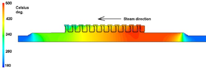
**Fig. 11 Thermal state of rotor and diaphragms of large steam turbine**
