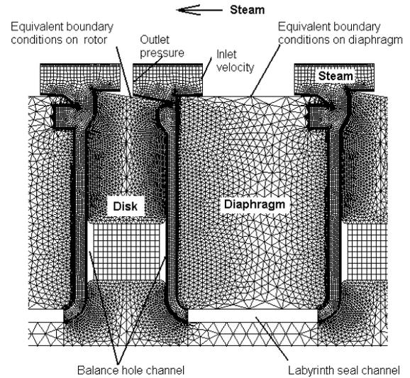
*Fig. 1 Fragment of the fluid-solid model for coupled analysis of thermal state of secondary flow in the high-pressure cylinder of large steam turbine*
