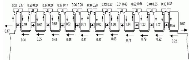
Fig. 7 Secondary steam relative mass flow rate vs. main steam flow
