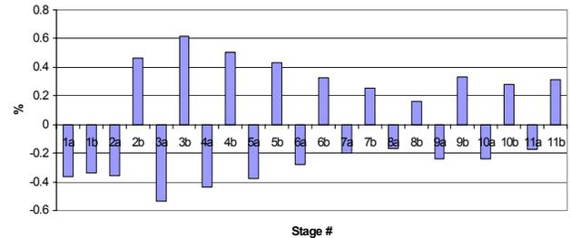
Fig. 6 Relative steam mass flow rate  $G_{leak}/G_{main}$  for suction (negative) and injection (positive) from/to flow path. Here 1a, 1b are the first and second cavities of the first disk, etc.
