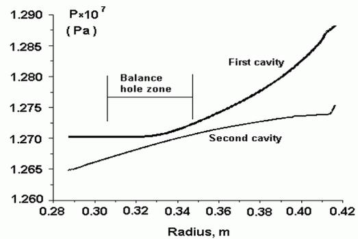
Fig. 5 Static pressure distribution in both near-to-disk cavities of the 4<sup>th</sup> stage
